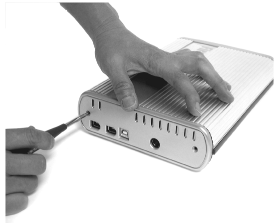
10. Install the Back Panel to the Enclosure and secure the Back Panel with two 5mm diameter screws.
