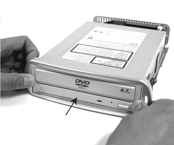
7. Push the Drive all the way into the Base Plate.
