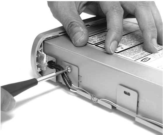
8. Secure the Drive to the Base Plate with four 7mm diameter screws on both side.
