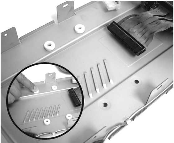
6. Align four white plastic spacers to the hole on the Base Plate and press the spacers to adhere.
