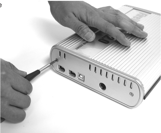
1. Unscrew two 5mm diameter screws to loosen the Back Panel.
