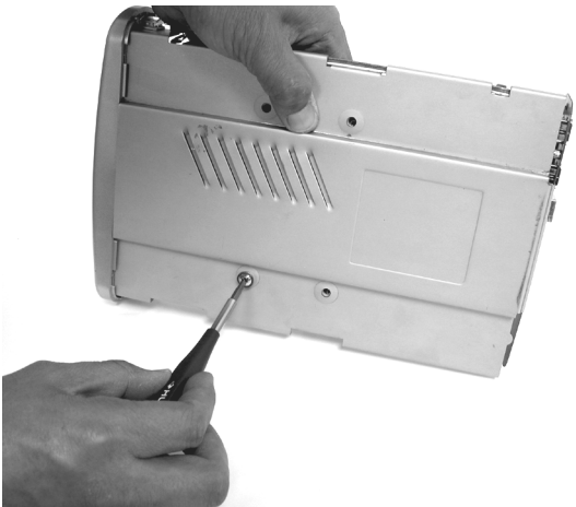
8. Align the hard drive and the Base Plate holes. Secure the Drive to Base Plate with four 10mm diameter screws.
