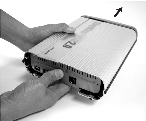
3. Use your thumb to push the Base Plate out.
