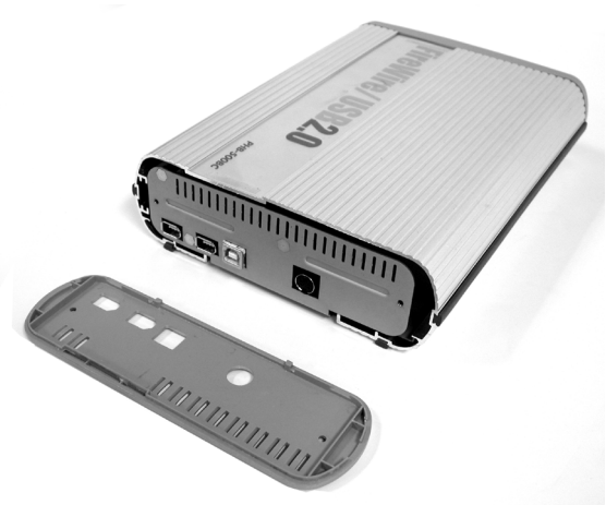
2. Remove the Back Panel from the Enclosure.
